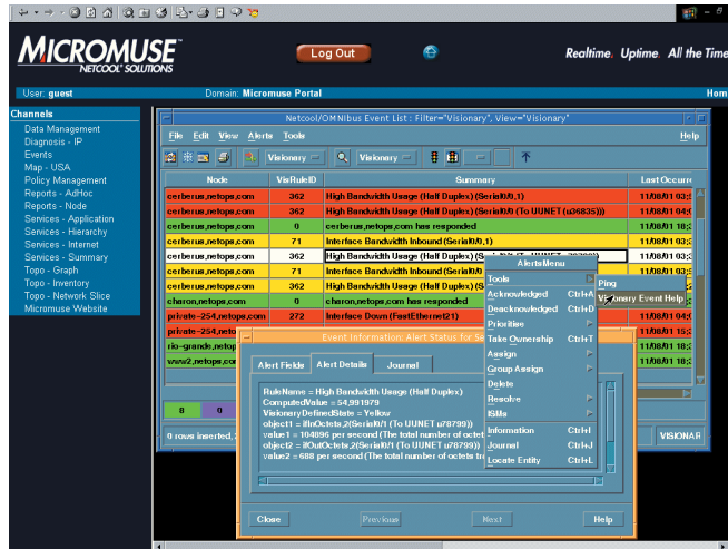
Netcool/Visionary problem diagnoses are reported alongside device status information in the Netcool EventList interface.
